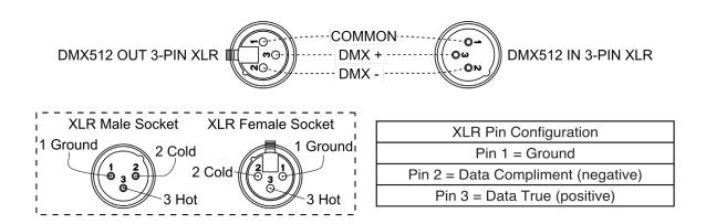
**Special Note: Line Termination.** When longer runs of cable are used, you may need to use a terminator on the last unit to avoid erratic behavior. A terminator is a 110-120 ohm 1/4 watt resistor which is connected between pins 2 and 3 of a male XLR connector (DATA + and DATA -). This unit is inserted in the female XLR connector of the last unit in your daisy chain to terminate the line. Using a cable terminator (ADJ part number Z-DMX/T) will decrease the possibilities of erratic behavior.
